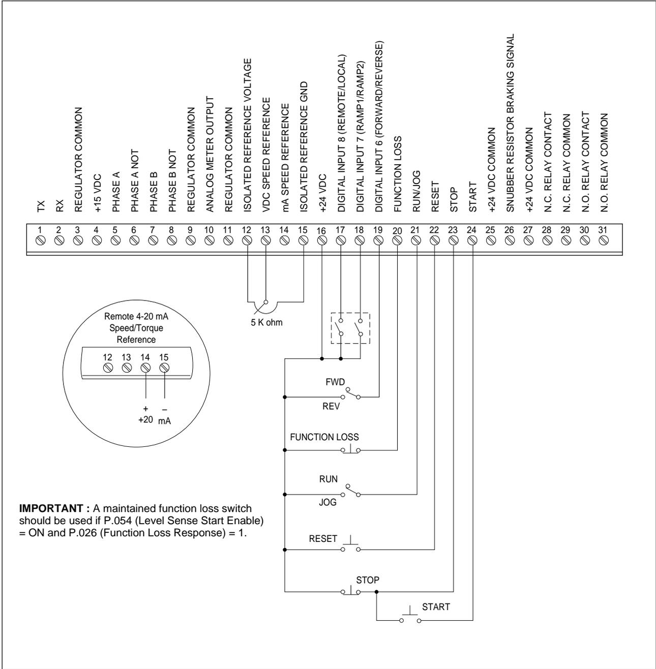
Figure 7.2 – Three-Wire Start/Stop Sample Control Wiring
