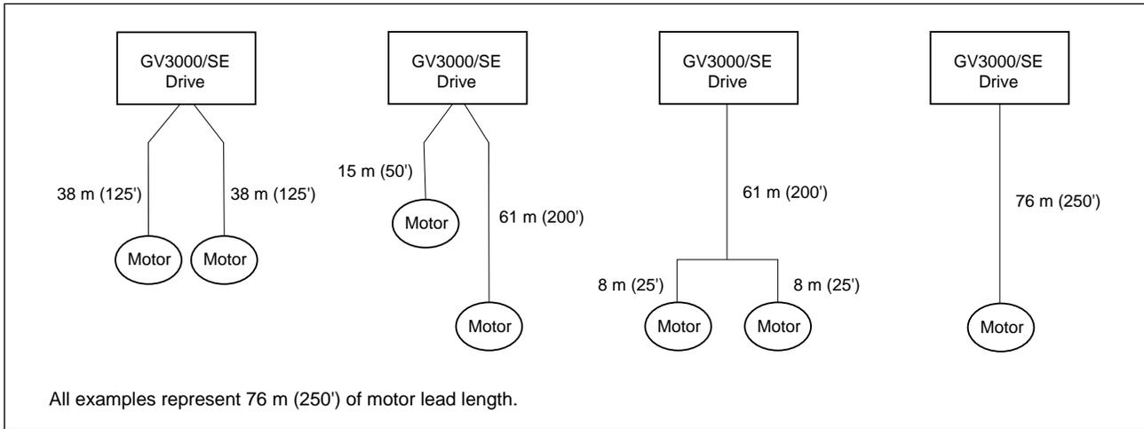
Figure 3.3 – How to Measure Motor Lead Lengths
