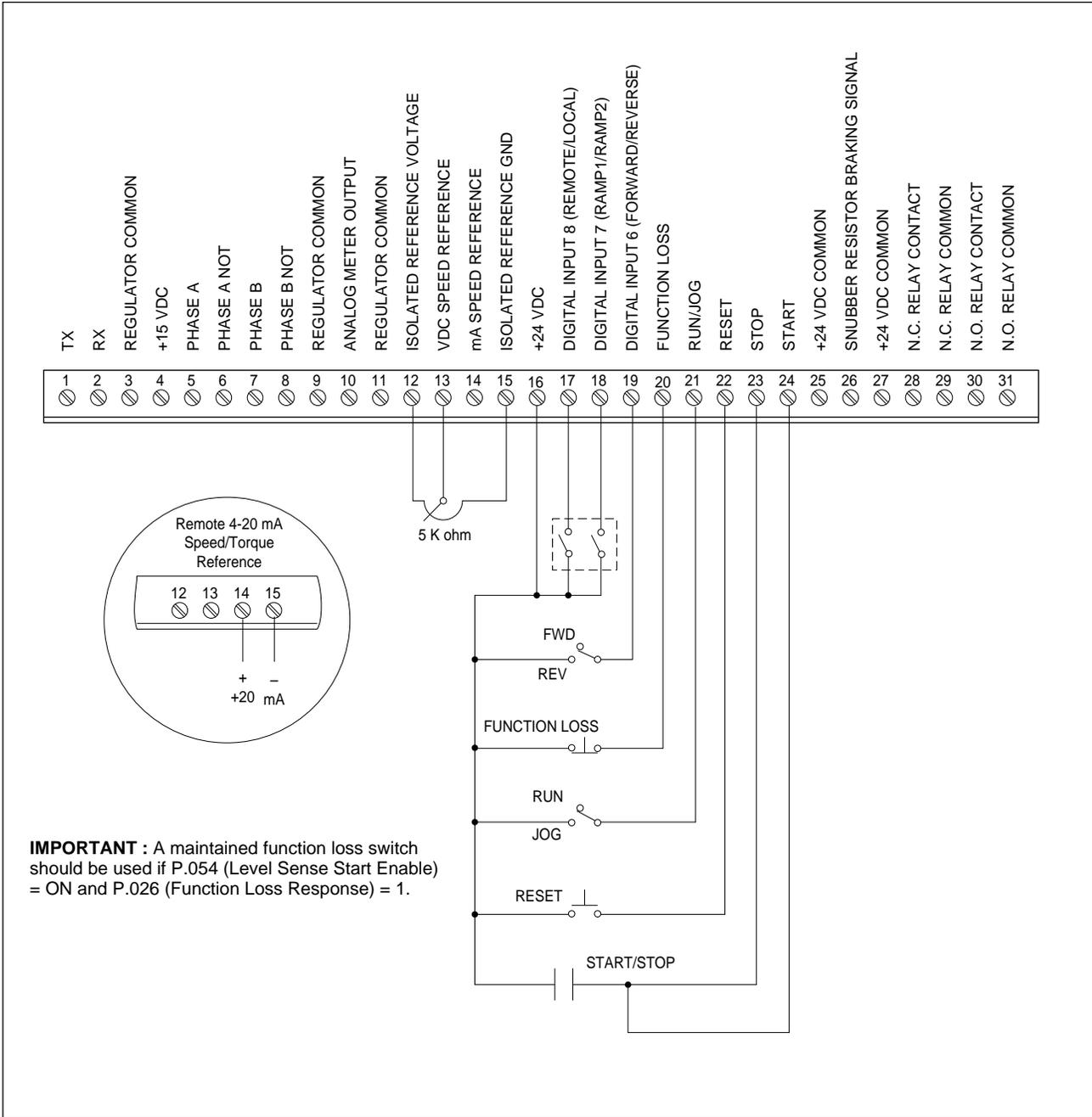
Figure 7.1 – Two-Wire Start/Stop Sample Control Wiring
