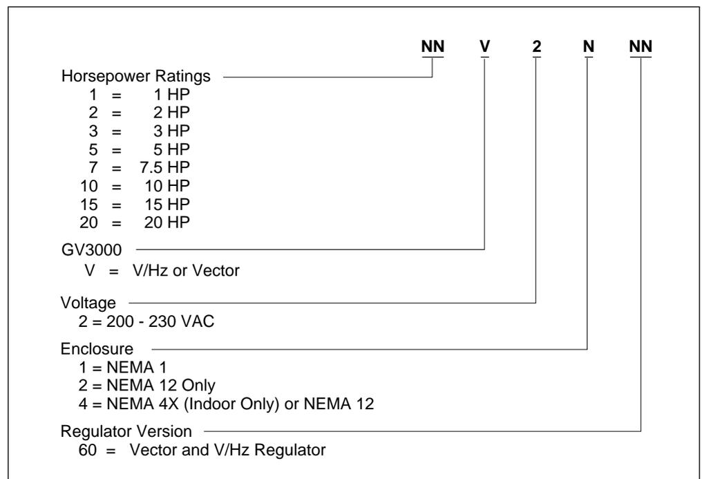
Figure 2.1 – Identifying the Drive Model Number
