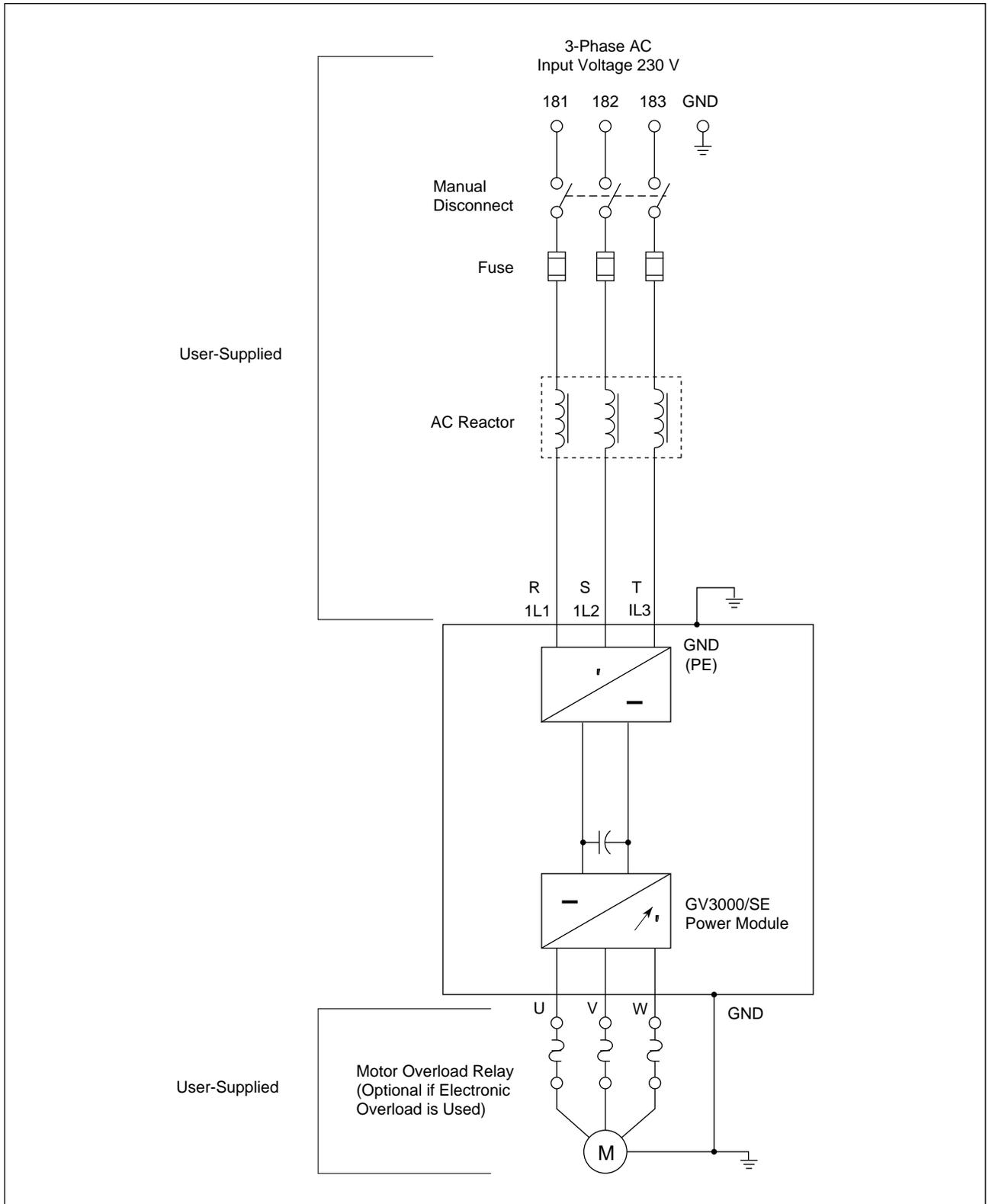
Figure 5.1 – Typical AC Input Electrical Connections
