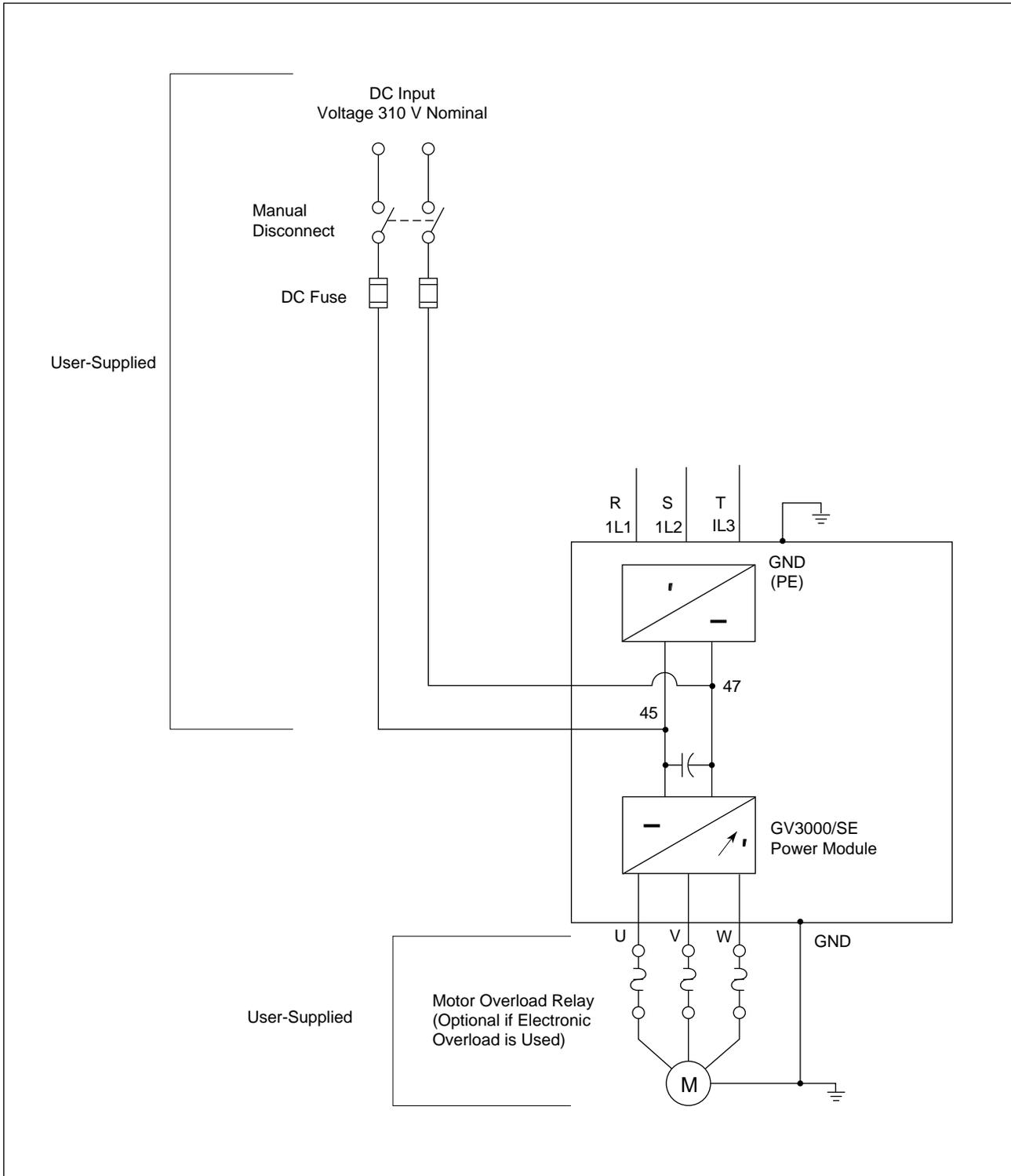
Figure 5.2 – Typical DC Bus Electrical Connections
