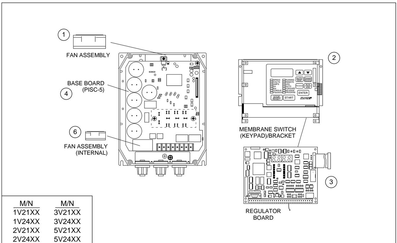
Figure 2.2 – 1 to 5 HP Drive Components and Locations
