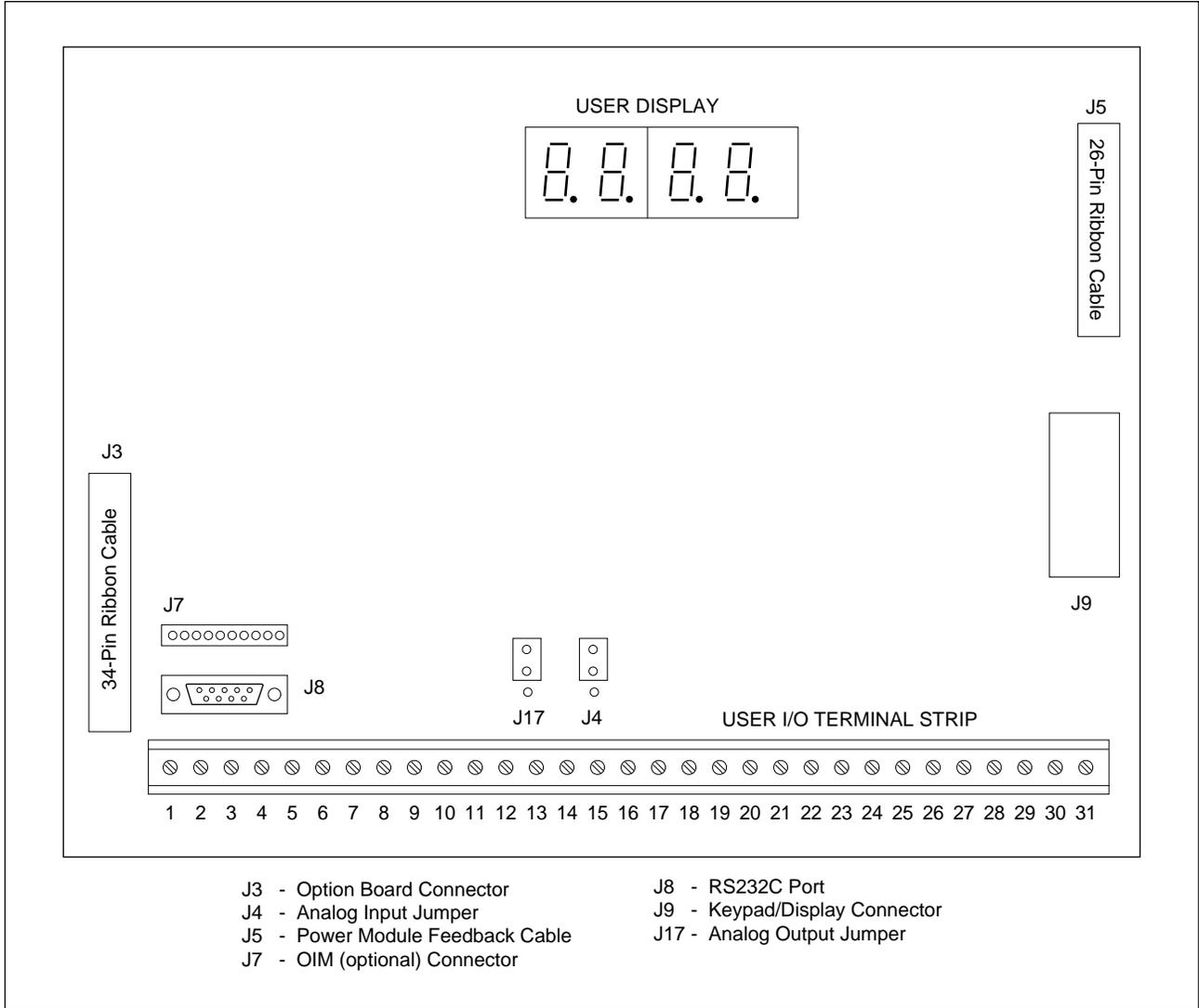
Figure 2.5 – Regulator Board Components and Locations
