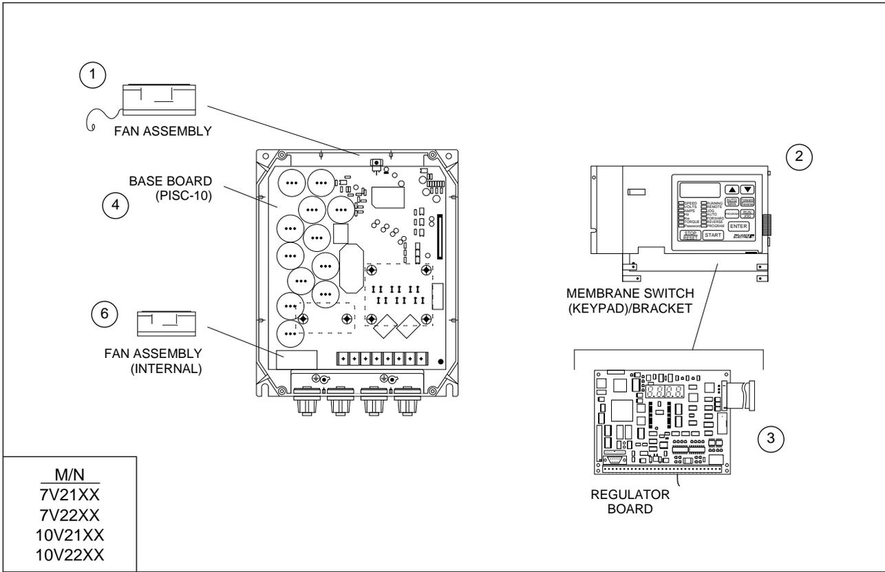
Figure 2.3 – 7.5 and 10 HP Drive Components and Locations
