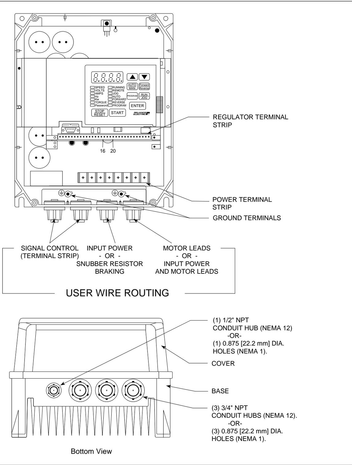
Figure 4.2 – Wire Routing Locations for 7.5 and 10 HP Drives
