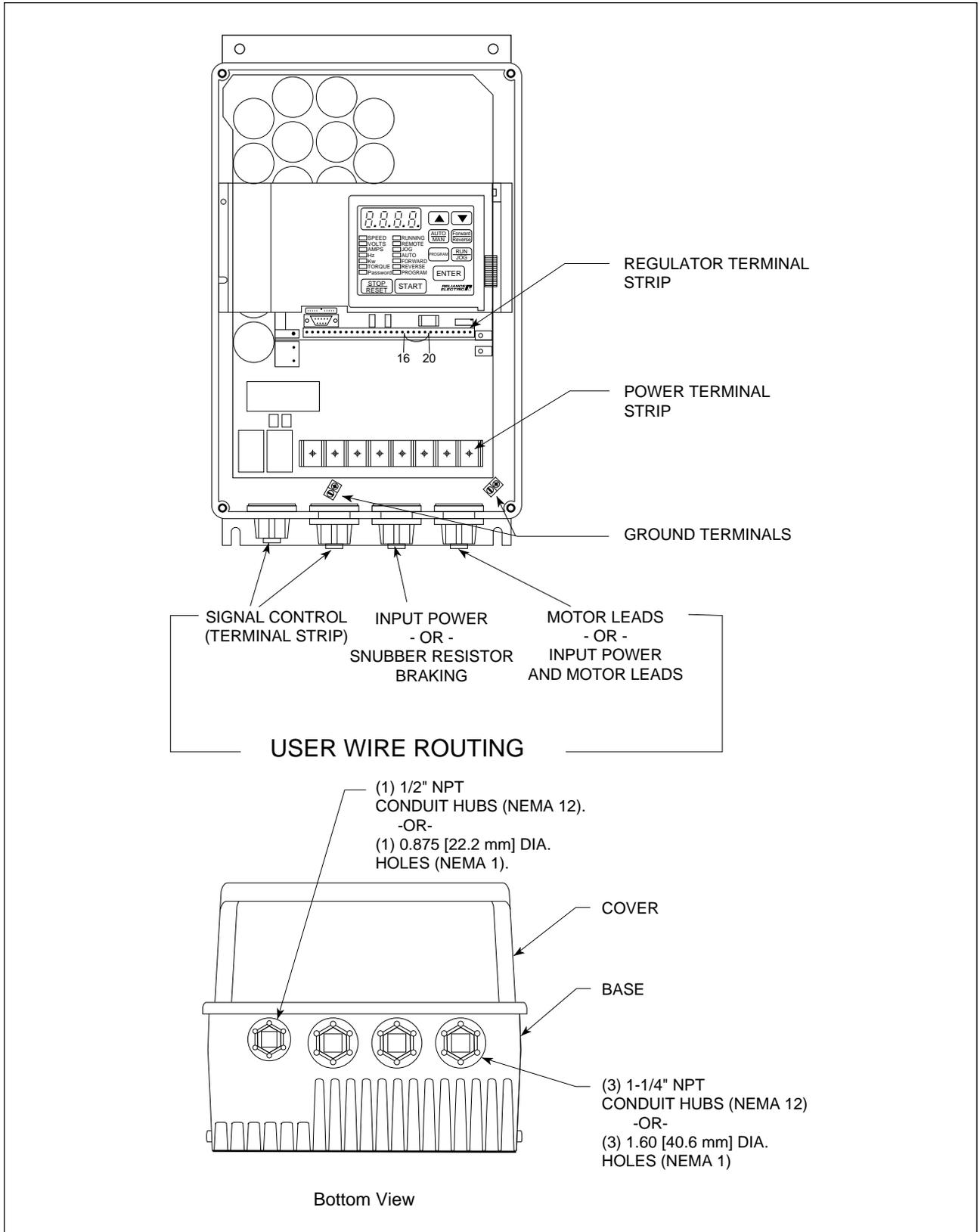
Figure 4.3 – Wire Routing Locations for 15 and 20 HP Drives
