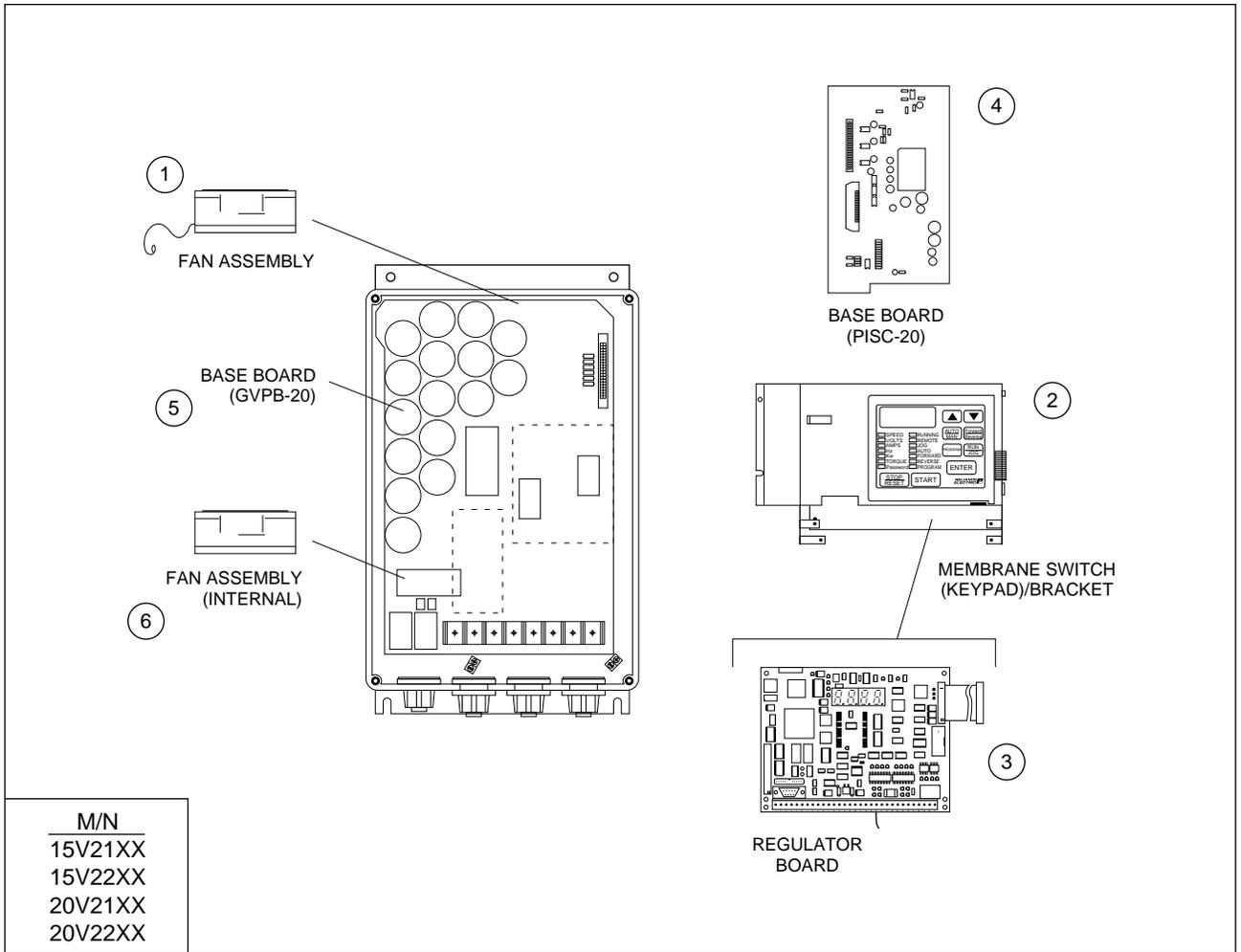
Figure 2.4 – 15 and 20 HP Drive Components and Locations
